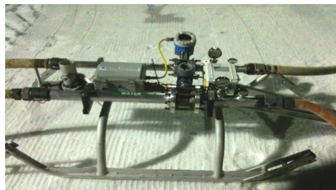
Snowmaking measurement sled with automated data collection for ease in measuring snow gun production versus energy use while monitoring conditions at which the snow is being made.
