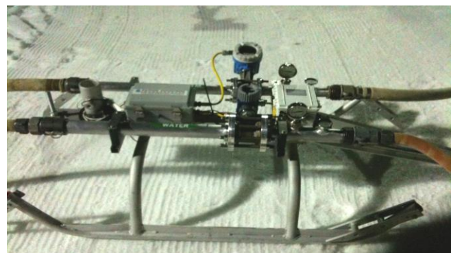
Snowmaking measurement sled with automated data collection for ease in measuring snow gun production versus energy use while monitoring conditions at which the snow is being made.
